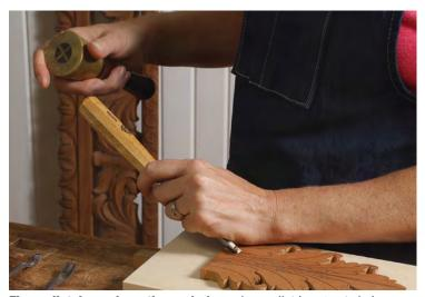
**The mallet depends on the work.** A wooden mallet is a great choice for heavy pounding, since it won't damage the gouge handle as readily as a metal one. A metal mallet of the same weight, though, is easier to grip around its head, making it better for gentler, nimbler taps.
