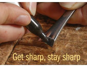
**Color the bevel with a Sharpie.** This lets you better monitor where the bevel is rubbing on the stones, especially the coarsest, helping you achieve an even surface.
