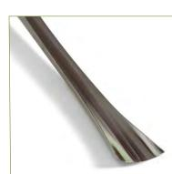
Fishtails have splayed corners. These gouges are May's favorite for detail work, since they are more slender than straight gouges and, more importantly, their sharp corners fit well into tight areas.
