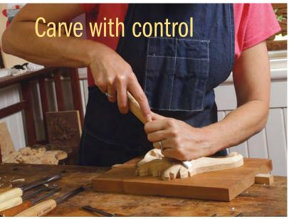
**Proper position.** Use both hands for maximum control and safety. One hand holds the handle to push the gouge; the other grips the metal shank to guide it. Brace this second hand against the wood for better control.
